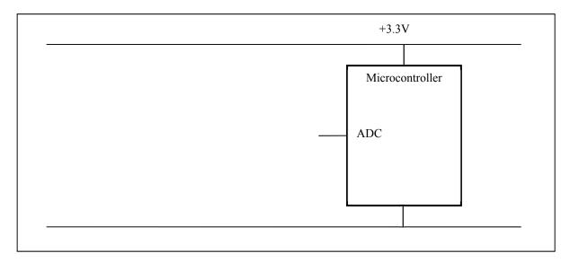
**b)** (10 points) The desired LED operating point is 1V, 10mA. Interface this LED to PA2 using *negative* logic. You can use any number of 7406 inverters, and any number of resistors. Assume the  $V_{OL}$  of the 7406 is 0.5V. Assume the microcontroller output voltages are  $V_{OH} = 3.1V$  and  $V_{OL} = 0.2V$ . Specify values for any resistors needed. Show equations of your calculations used to select resistor values.
