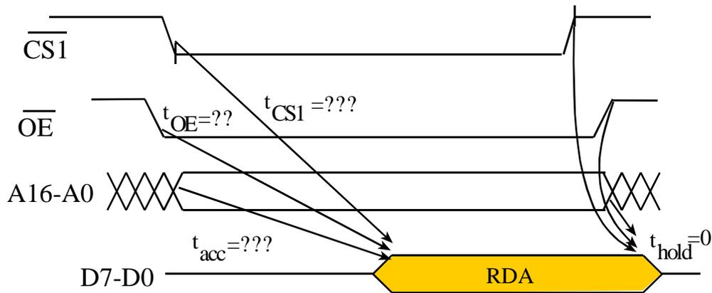
Figure 9.1. Read timing for the 128K RAM chip.
