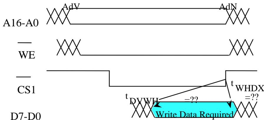
Figure 9.2. Write timing controlled by  $\overline{CS1}$ .
