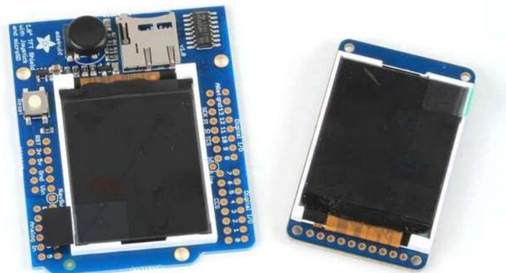
The 1.8" display has 128x160 color pixels. Unlike the low cost "Nokia 6110" and similar LCD displays, which are CSTN type and thus have poor color and slow refresh, this display is a true TFT! The TFT driver (ST7735R) can display full 18-bit color (262,144 shades!). And the LCD will
