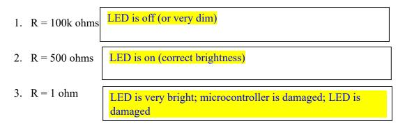
(5) Part c) Suppose the desired operating point of the diode is 1.7V, 3mA. The high voltage of the microcontroller is 3.1V, and the low voltage of the microcontroller is 0.1V. Derive an equation and solve for the correct R?
