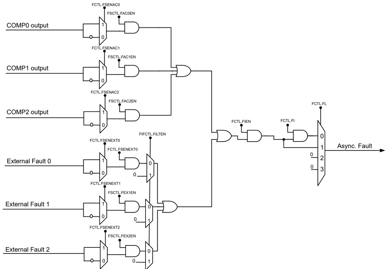
Figure 23-34. Asynchronous Fault Handler Connections
