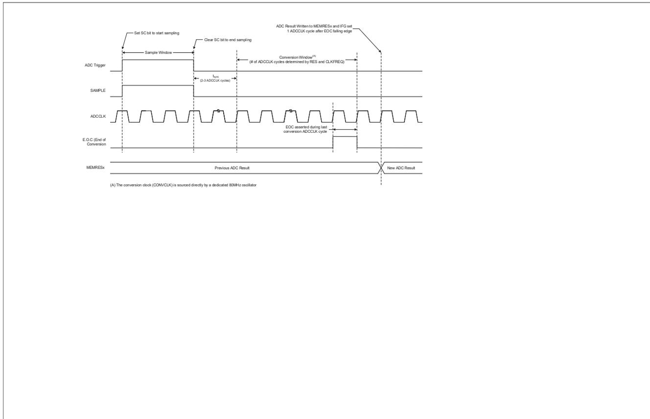
**Figure 10-3. MANUAL Sampling Mode ADC Sample and Conversion Timing Diagram**
