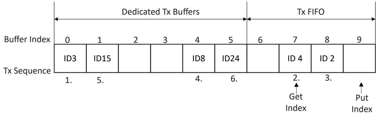
**Figure 19-14. Mixed Dedicated Tx Buffers/ Tx FIFO (example)**
