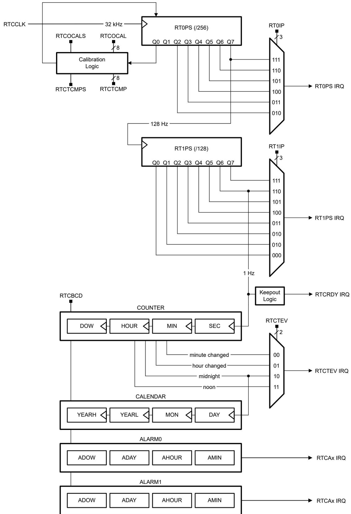
Figure 24-1. RTC Block Diagram
