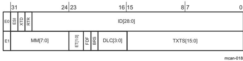
**Figure 19-23. Tx Event FIFO Element Structure**
