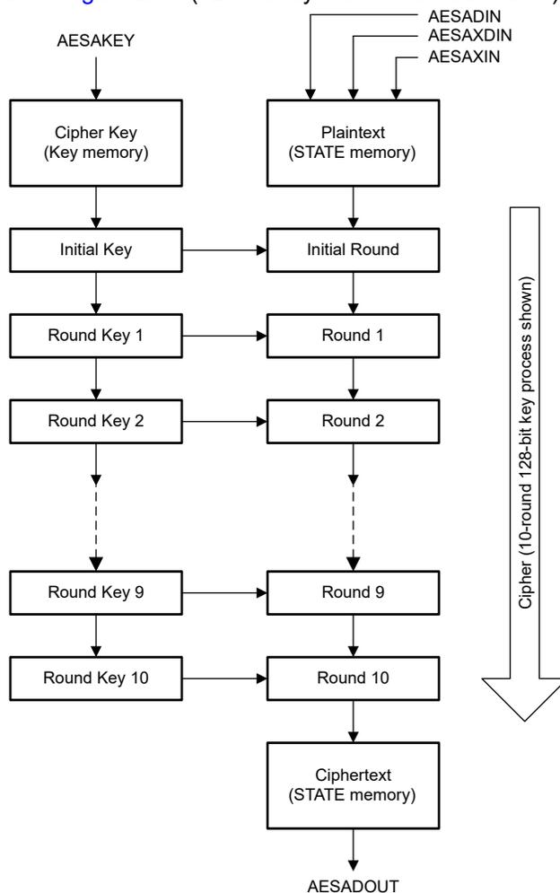
**Figure 21-3. AES Encryption (OPx=0x0, 128-bit Key)**
