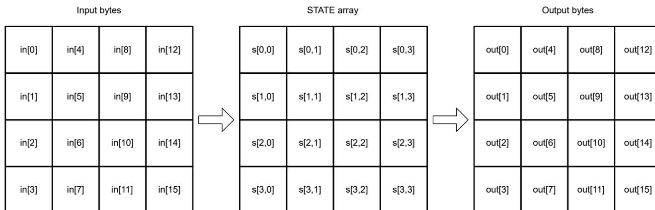
**Figure 21-2. AES State Array Input and Output**
