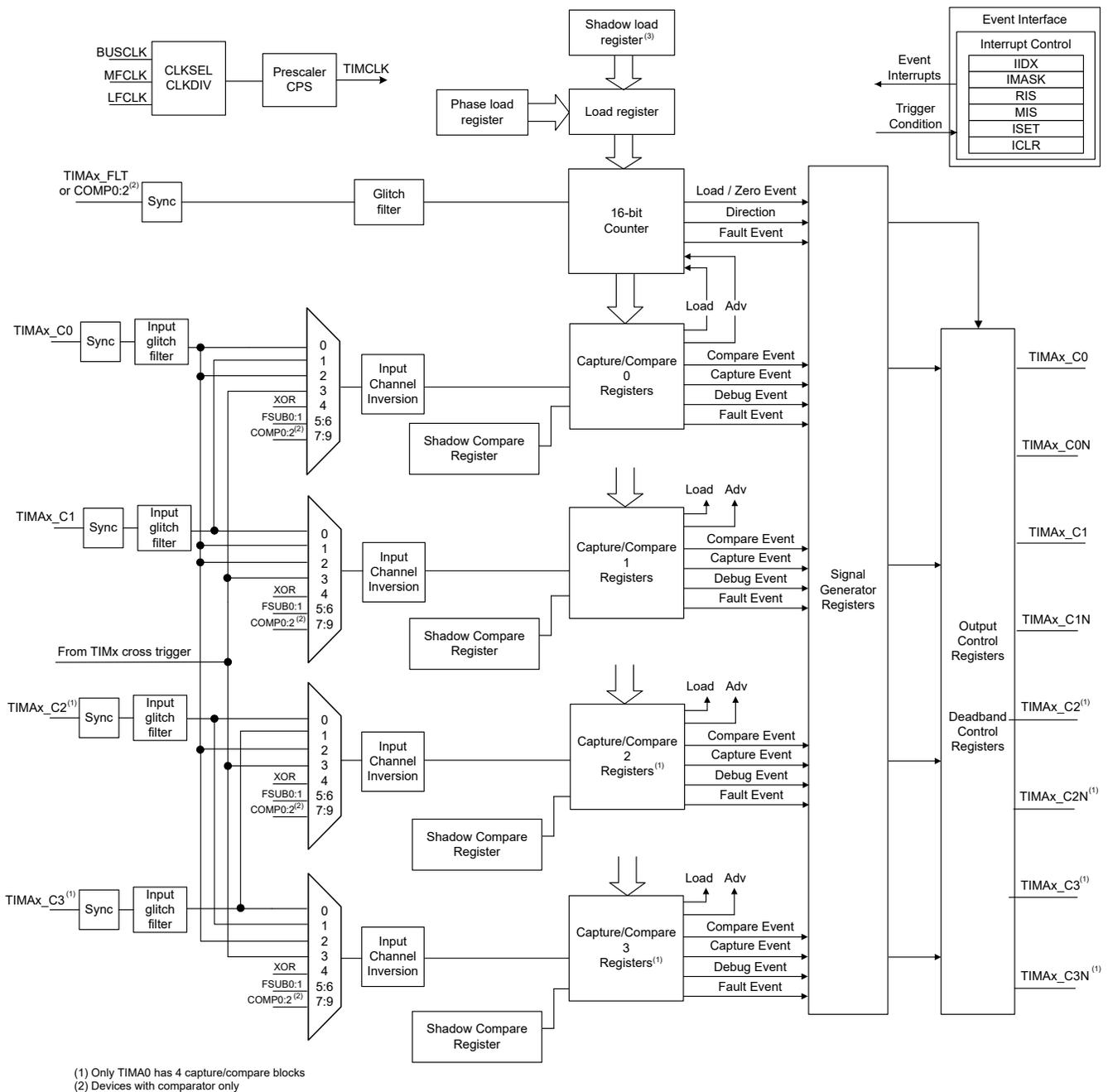
Figure 23-2. TIMA Block Diagram
