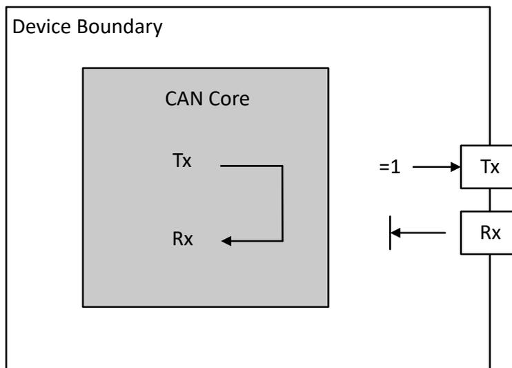
**Figure 19-12. Internal Loop Back Mode**
