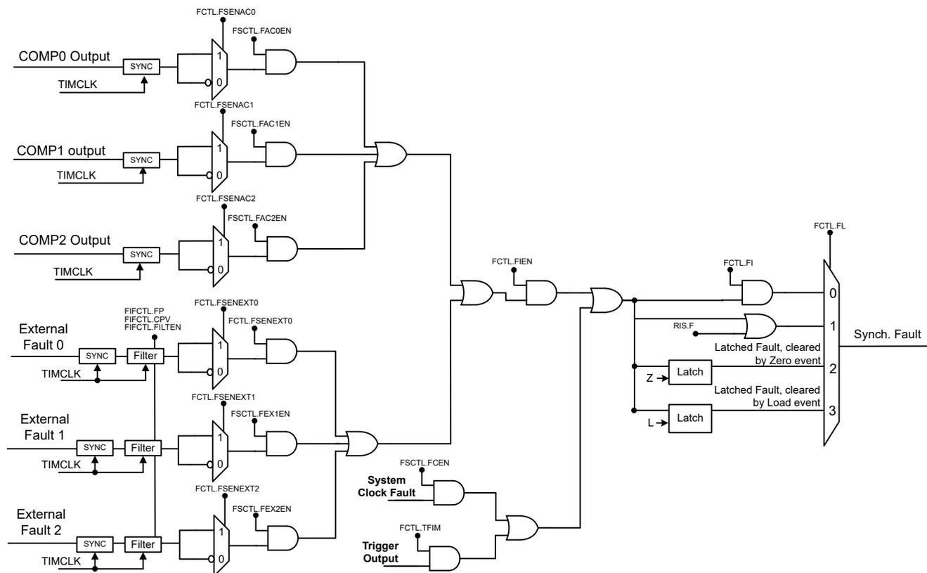
Figure 23-35. Synchronous Fault Handler Connections
