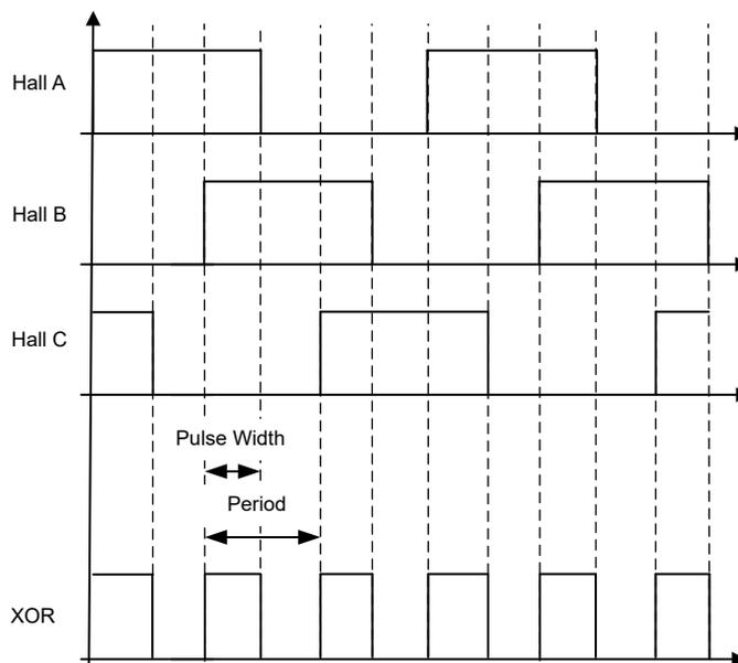
**Figure 23-22. Hall 3-Input XOR Signal used with Pulse Width or Period Capture for Speed Computation**
