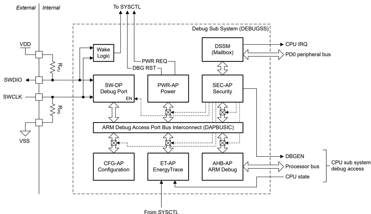
**Figure 26-1. Debug Sub System Block Diagram**
