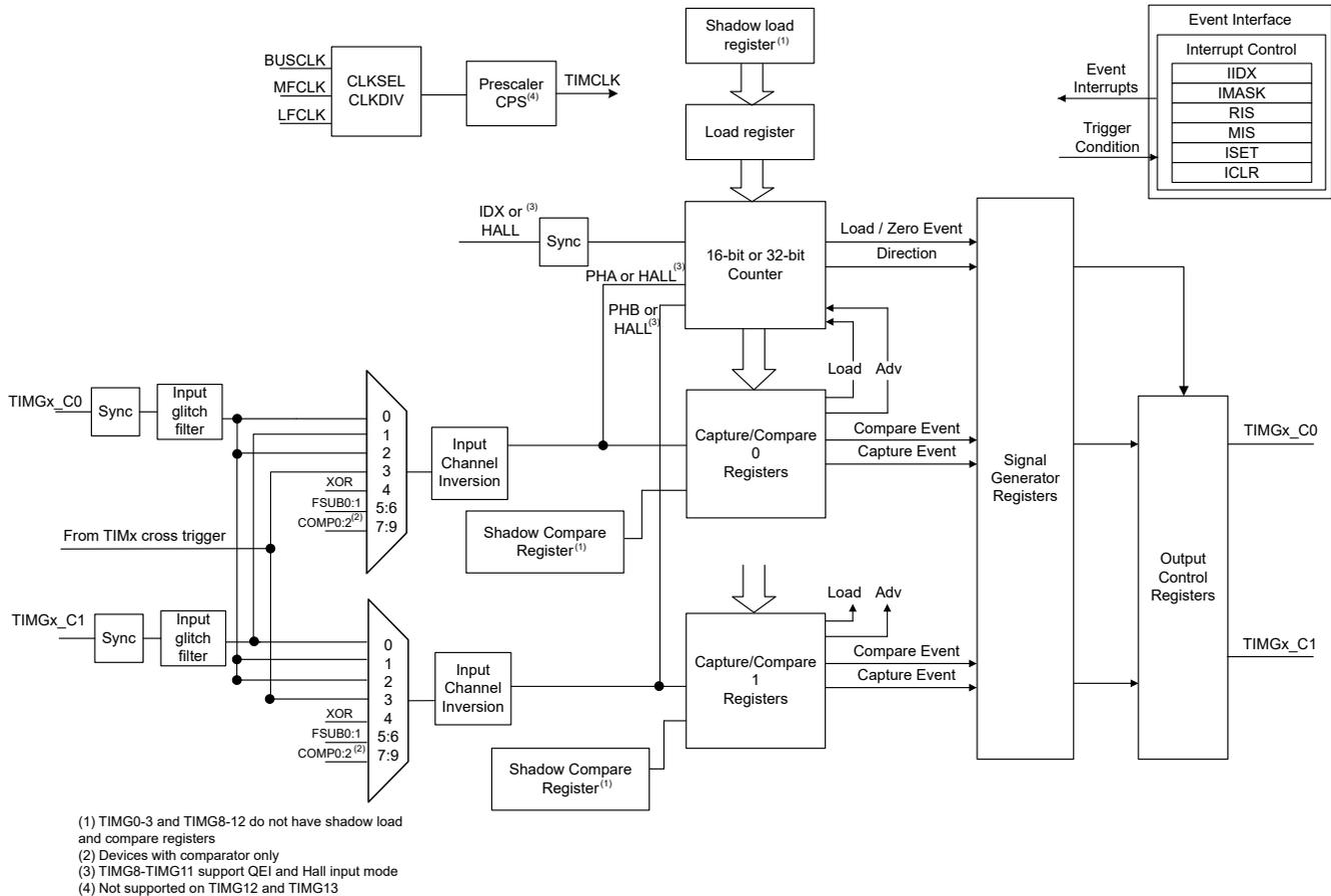
Figure 23-1. TIMx Functional Block Diagram
