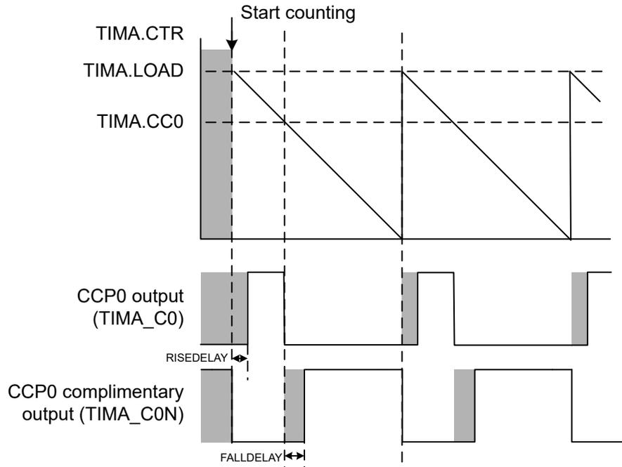
**Figure 23-32. Deadband Insertion for Edge-Aligned PWM in Down-Counting Mode using TIMA CC output channel 0 (M1\_ENABLE = 0)**
