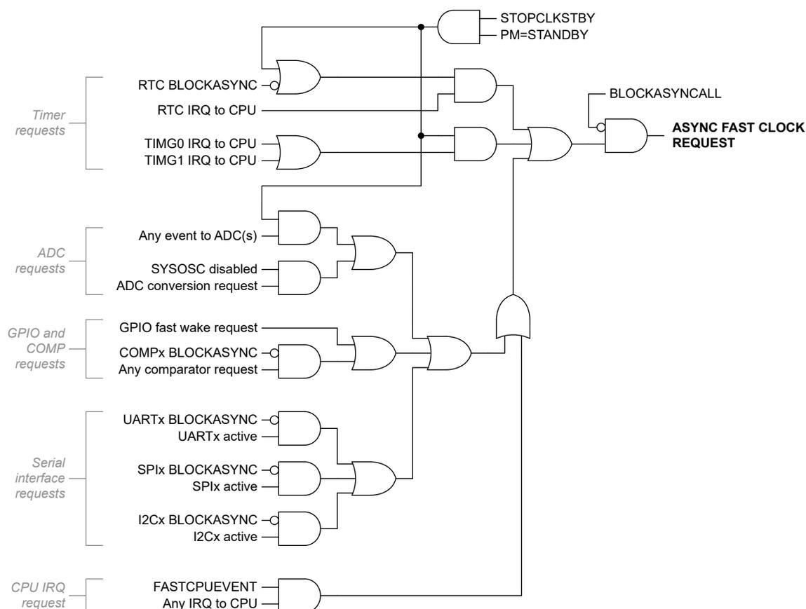
**Figure 2-11. MSPM0Gxx Asynchronous Fast Clock Request Logic**
