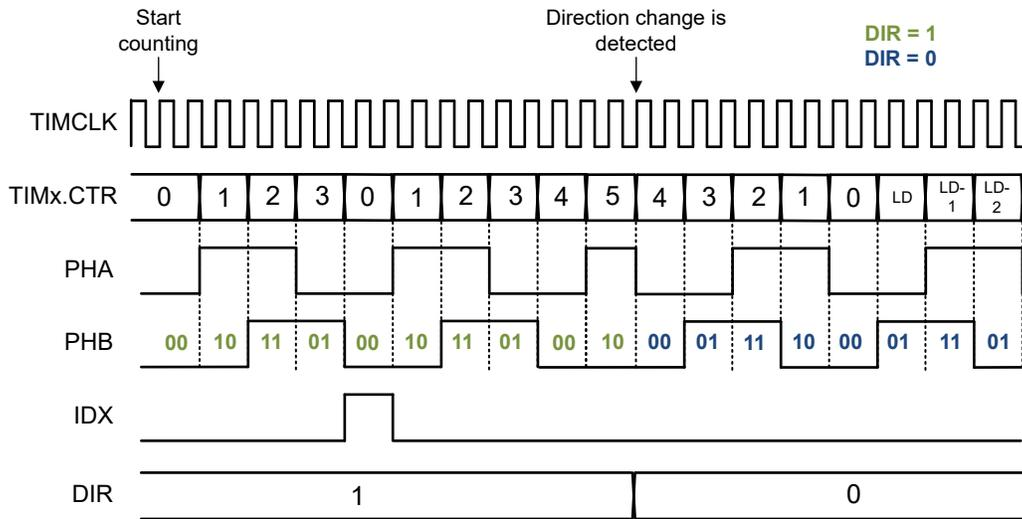
Figure 23-20. 2-Signal QEI with Index Input Operation
