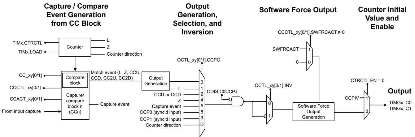
Figure 23-26. Output Connection for TIMG
