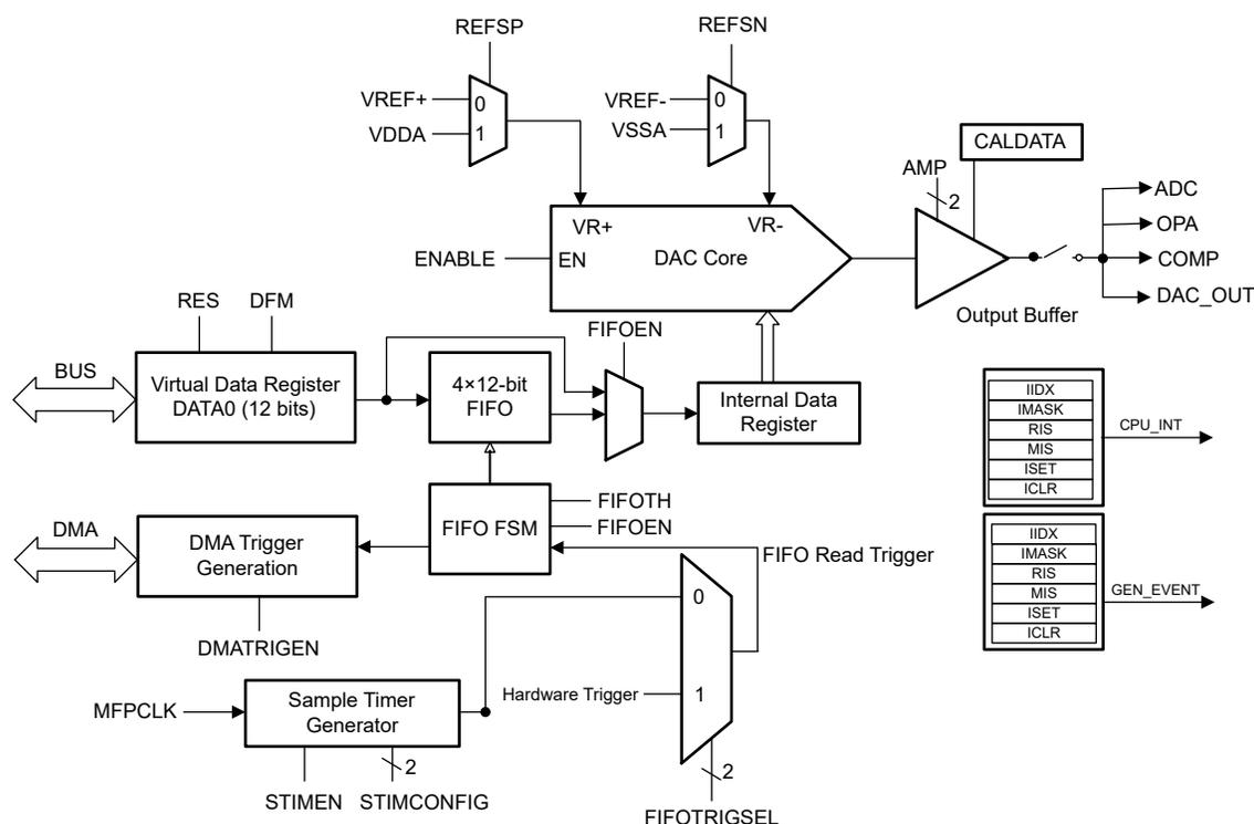
Figure 14-1. DAC Block Diagram
