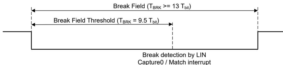
**Figure 16-5. LIN Break Field Detection**
