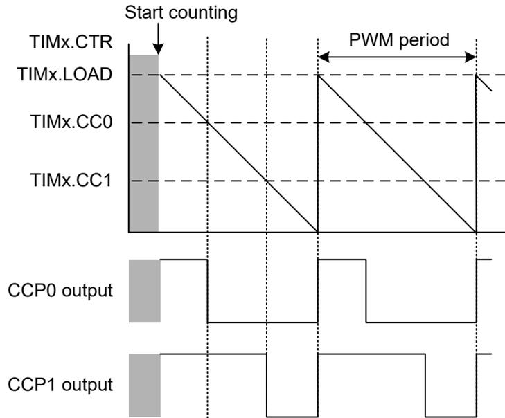
**Figure 23-28. Edge-Aligned PWM Signals in Down-Counting Mode**
