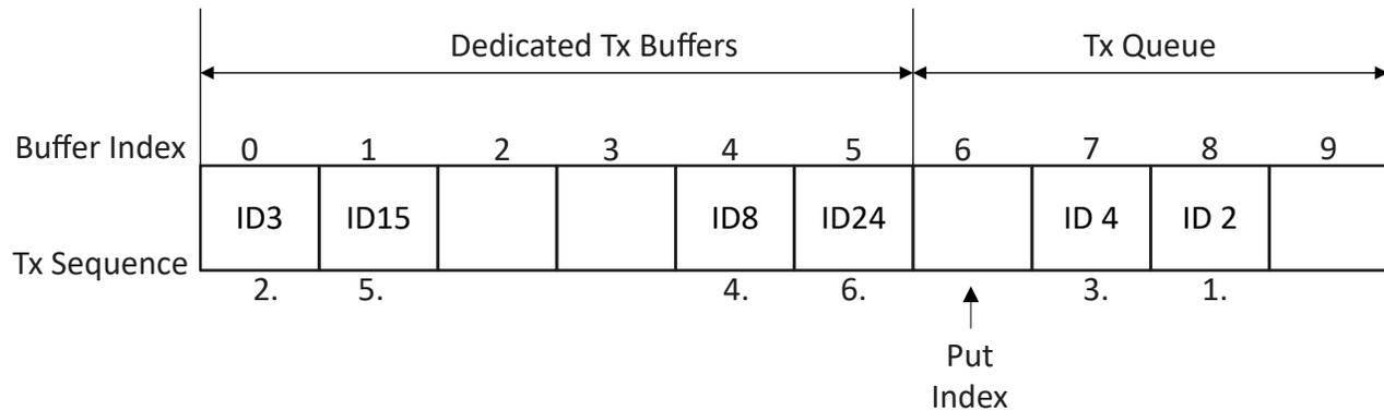
**Figure 19-15. Mixed Dedicated Tx Buffers/ Tx FIFO (Example)**
