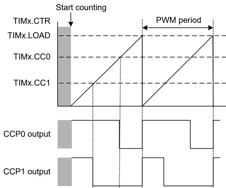
**Figure 23-29. Edge-Aligned PWM Signals in Up-Counting Mode**
