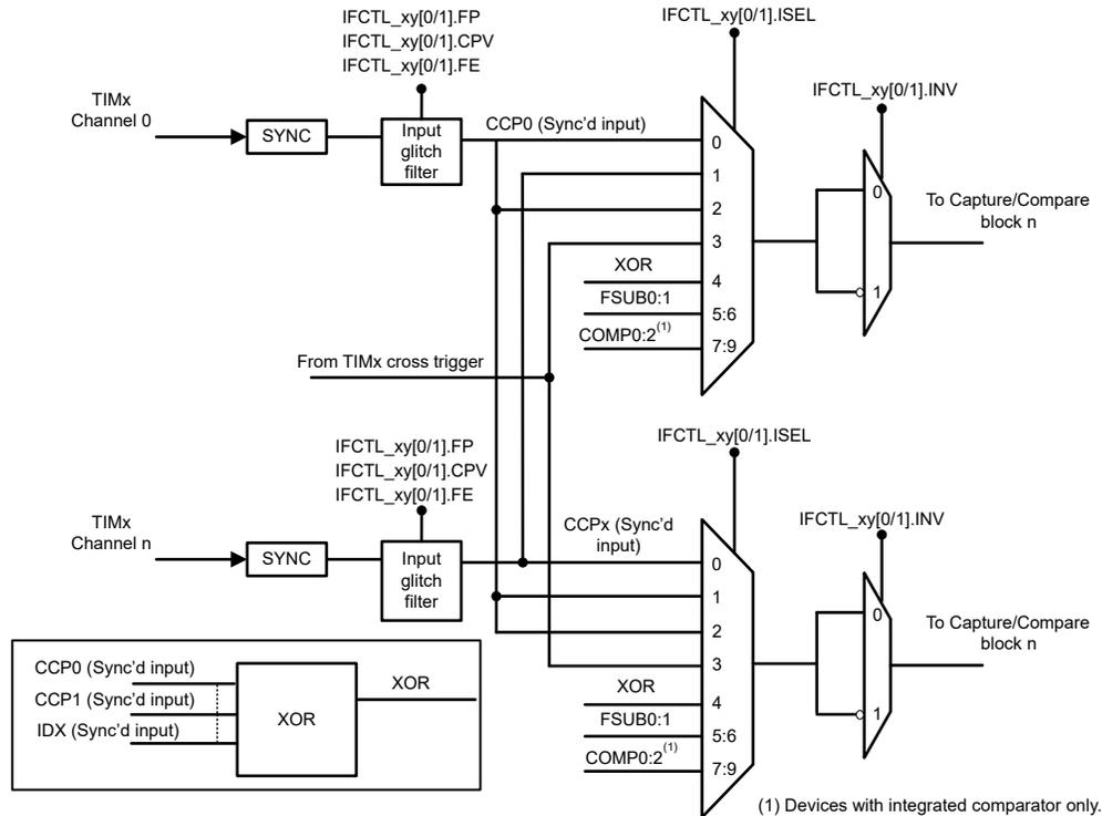
Figure 23-12. TIMx Capture Block Diagram
