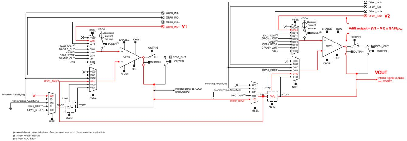
Figure 12-8. Two OPAs in Difference Amplifier Configuration
