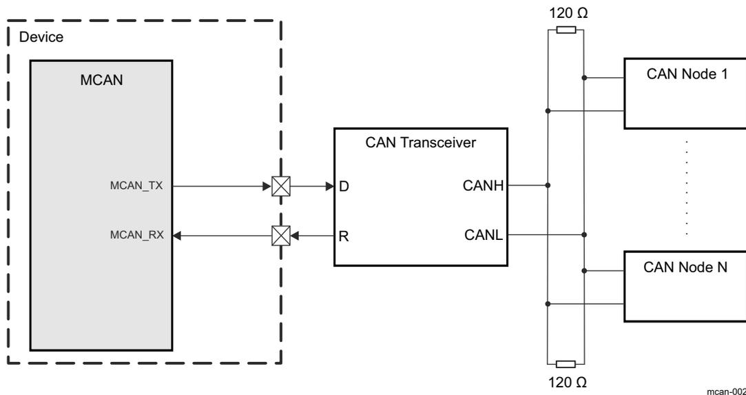
**Figure 19-2. MCAN Typical Bus Wiring**
