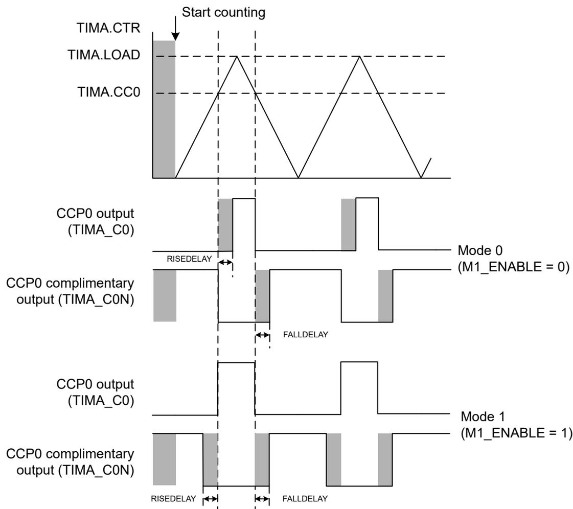
**Figure 23-33. Dead Band Insertion for Center-Aligned PWM (Mode 0 and Mode 1)**
