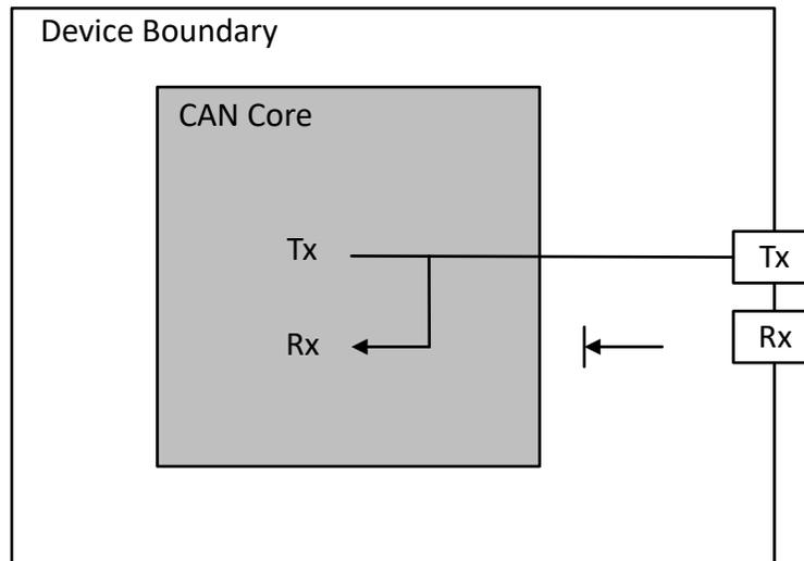
Figure 19-11. External Loop Back Mode
