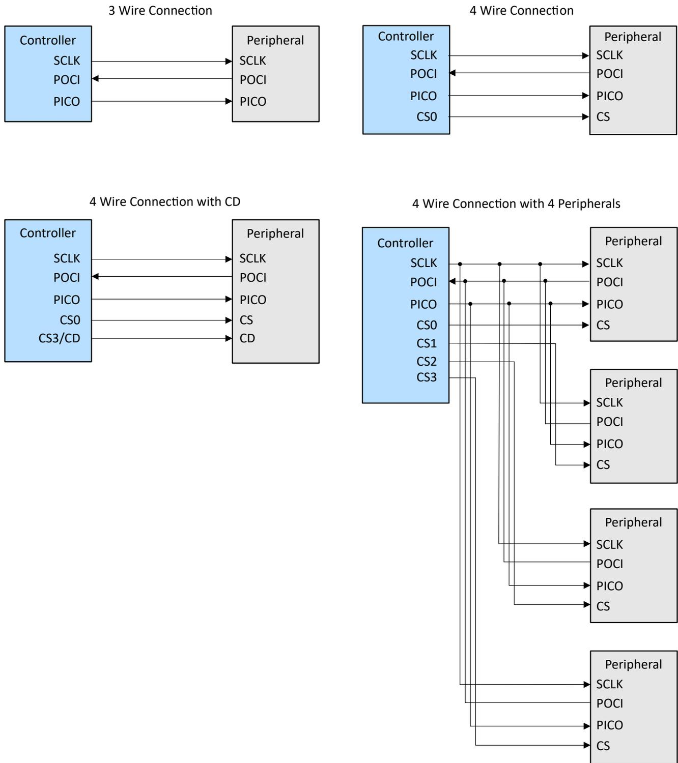
**Figure 17-2. External Connections for Different SPI Configurations**
