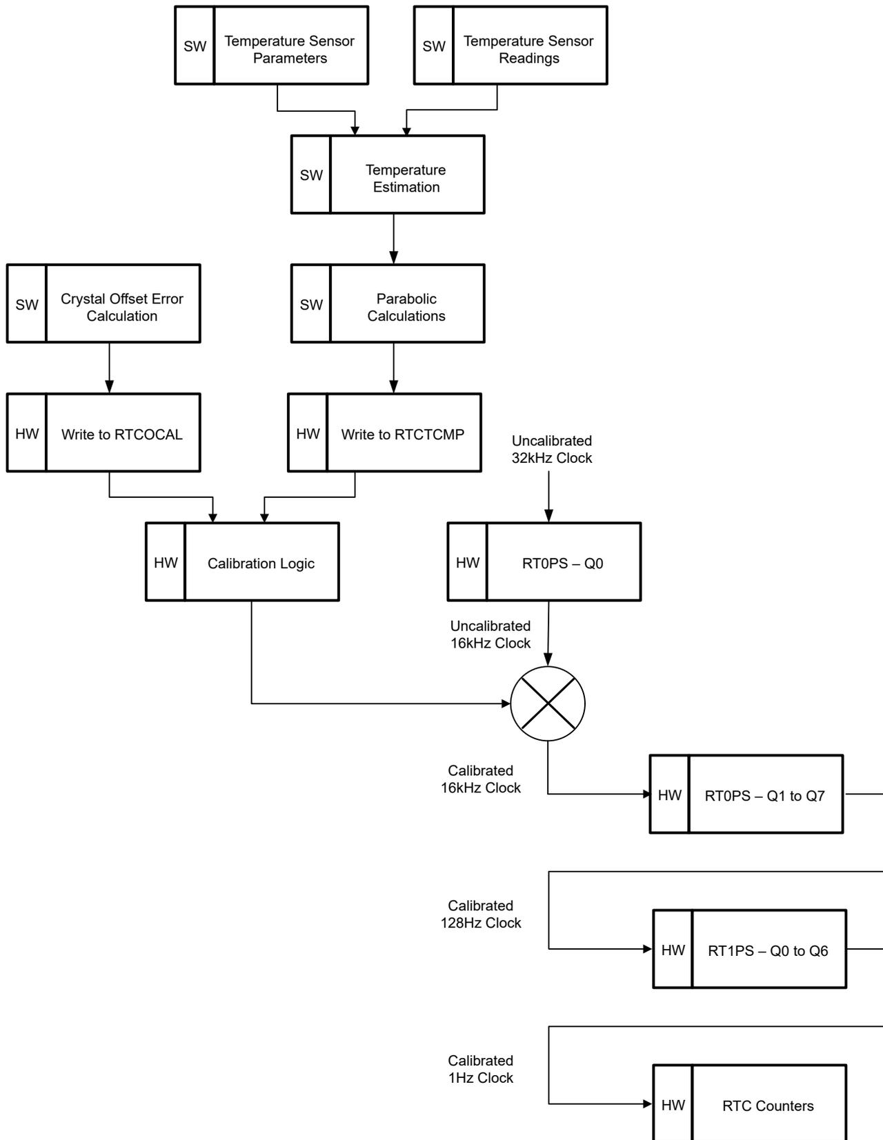
Figure 24-2. RTC Calibration
