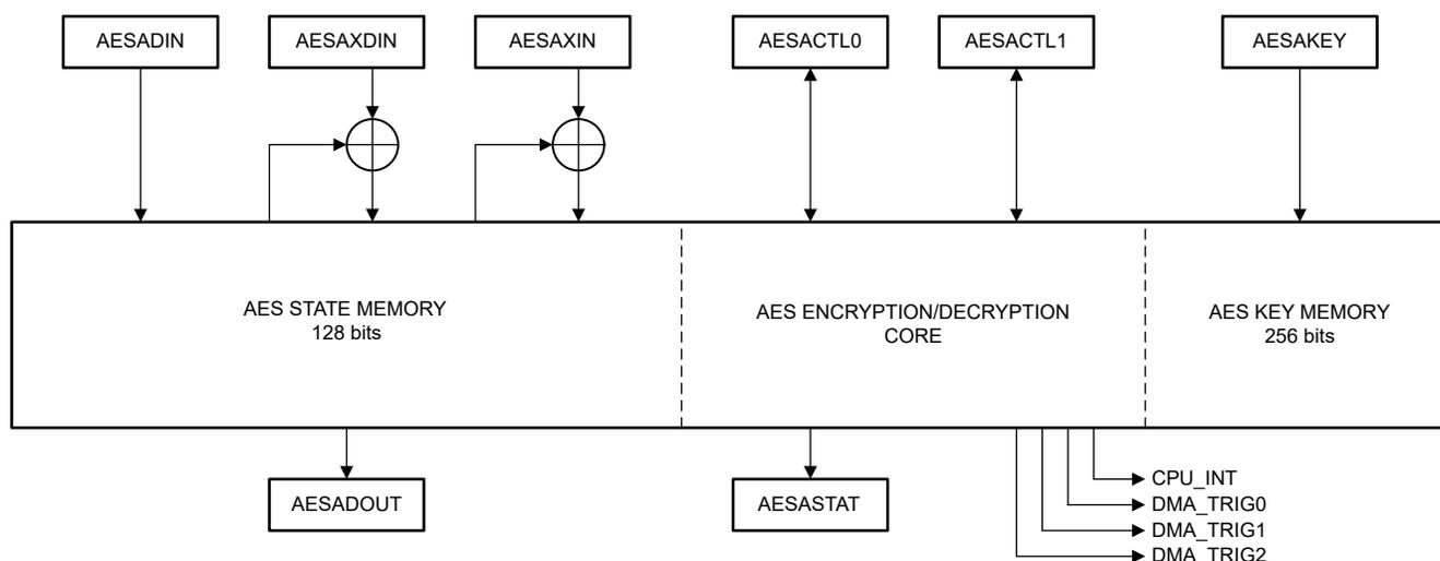
**Figure 21-1. AES Accelerator Block Diagram**
