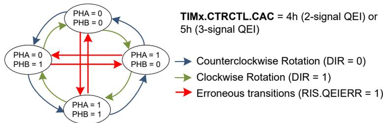
**Figure 23-18. State Machine for 2-signal and 3-signal QEI mode**
