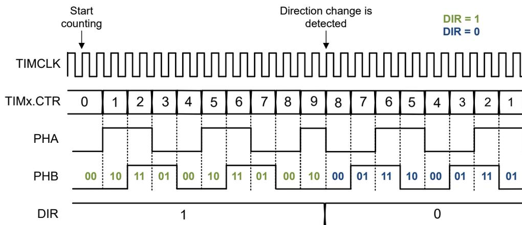
**Figure 23-19. 2-Signal QEI Operation**
