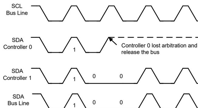
**Figure 18-8. Arbitration Procedure Between Two Controller Transmitters**
