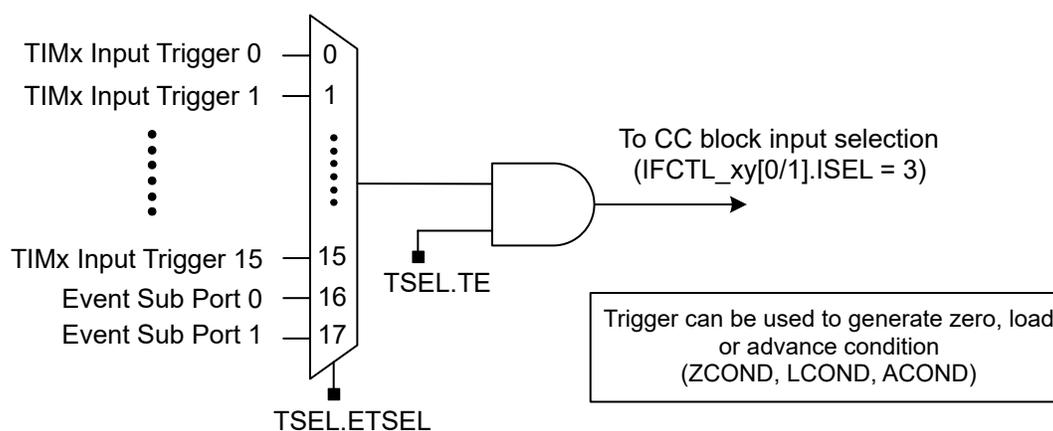
**Figure 23-40. Secondary Timer Cross Trigger Input Configuration**
