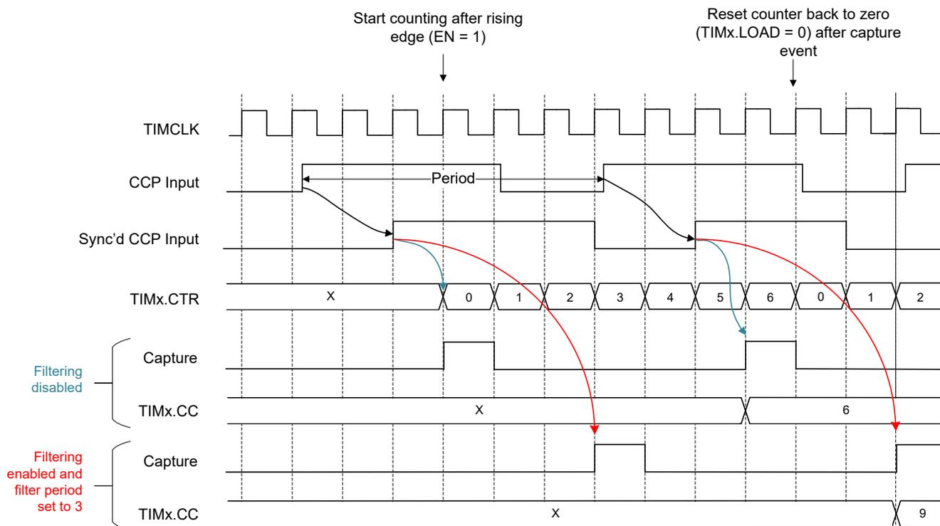
**Figure 23-15. Period Capture Mode in Up-Counting Mode, CVAE = 2**
