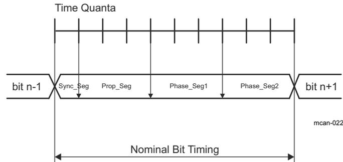
**Figure 19-5. CAN Bit Timing**
