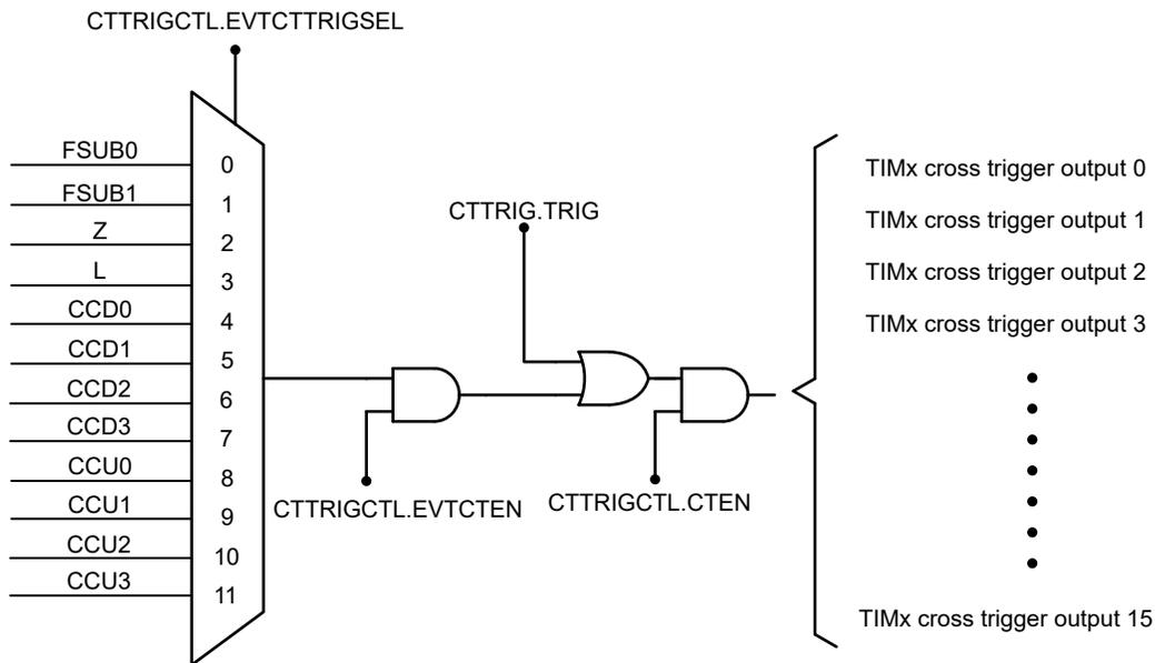
**Figure 23-39. Main Timer Cross Trigger Output Configuration**
