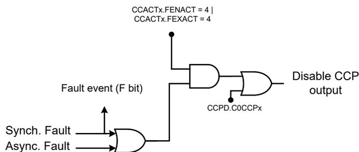
Figure 23-36. Fault Output Generation Connections
