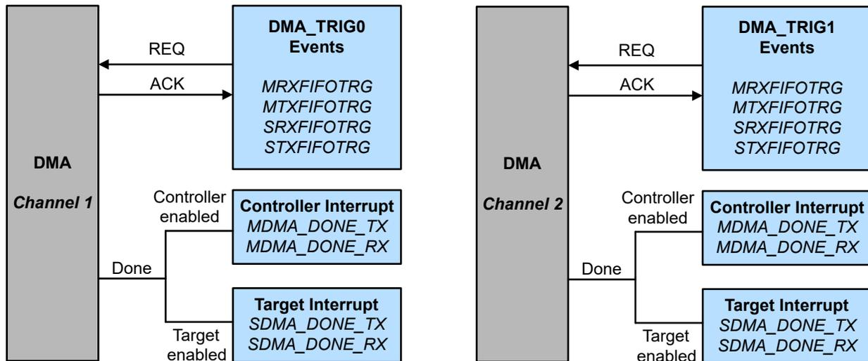
Figure 18-17. I<sup>2</sup>C DMA Trigger and Status
