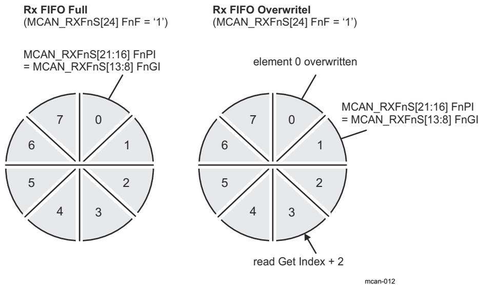
**Figure 19-19. Rx FIFO Overflow Handling**
