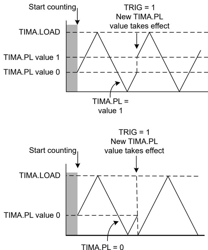
**Figure 23-11. Phase Load Register Synchronization in Up-Down Mode**
