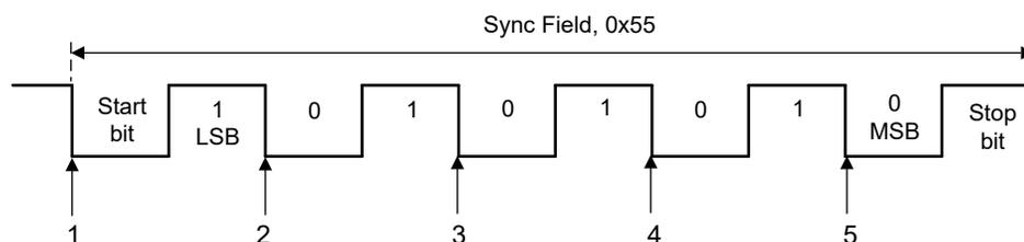
**Figure 16-6. LIN SYNC Field Detection**
