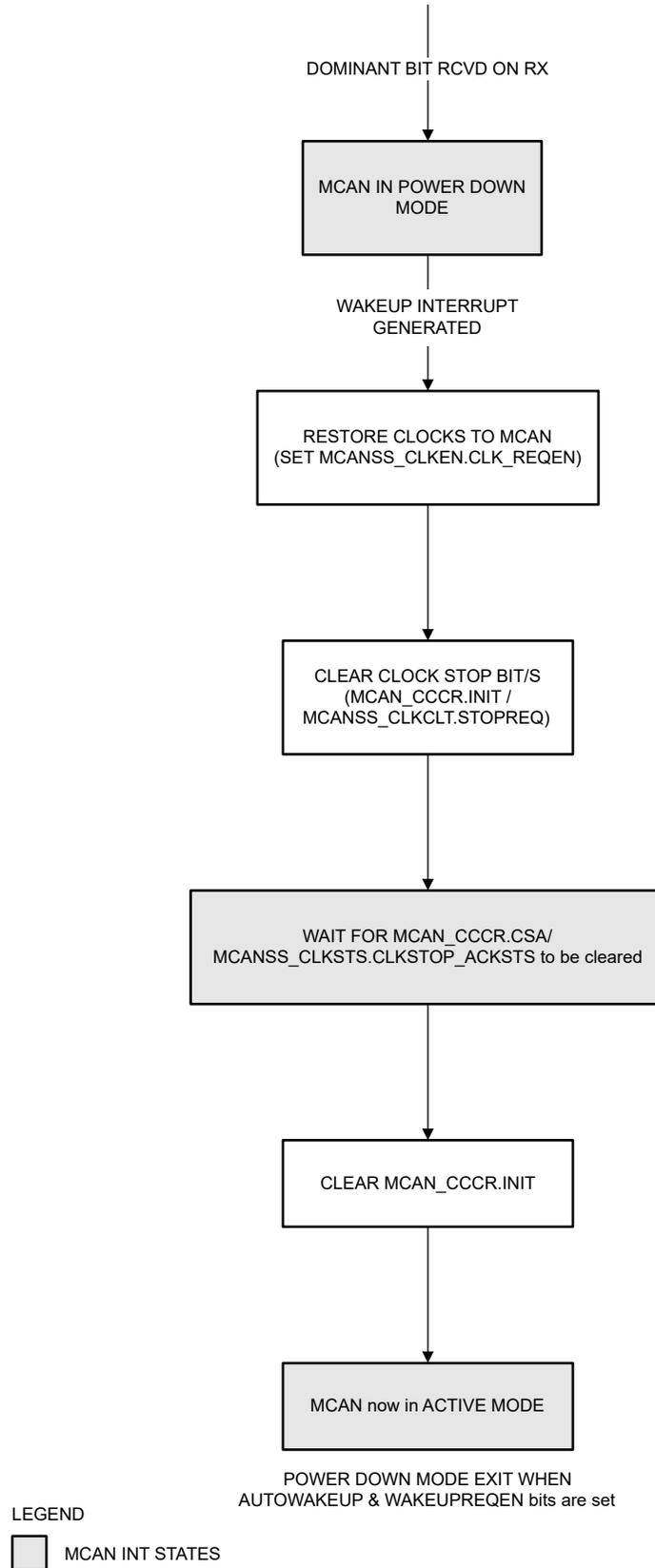
**Figure 19-10. Auto Wakeup Enabled Exit from Power Down**
