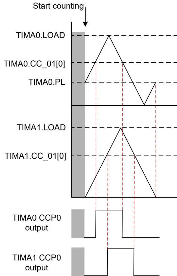
**Figure 23-31. Asymmetric PWM Configuration with Phase Load for CCP channel 0 of TIMA0 and TIMA1**
