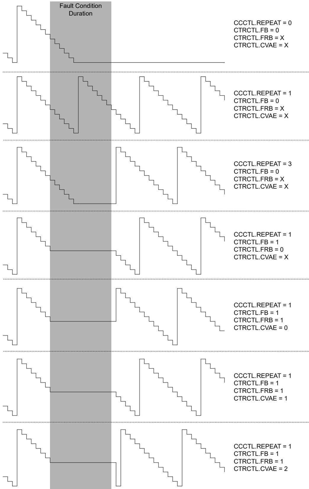
**Figure 23-37. Counter Behavior in Fault Condition with TIMx.CTRCTL Register**
