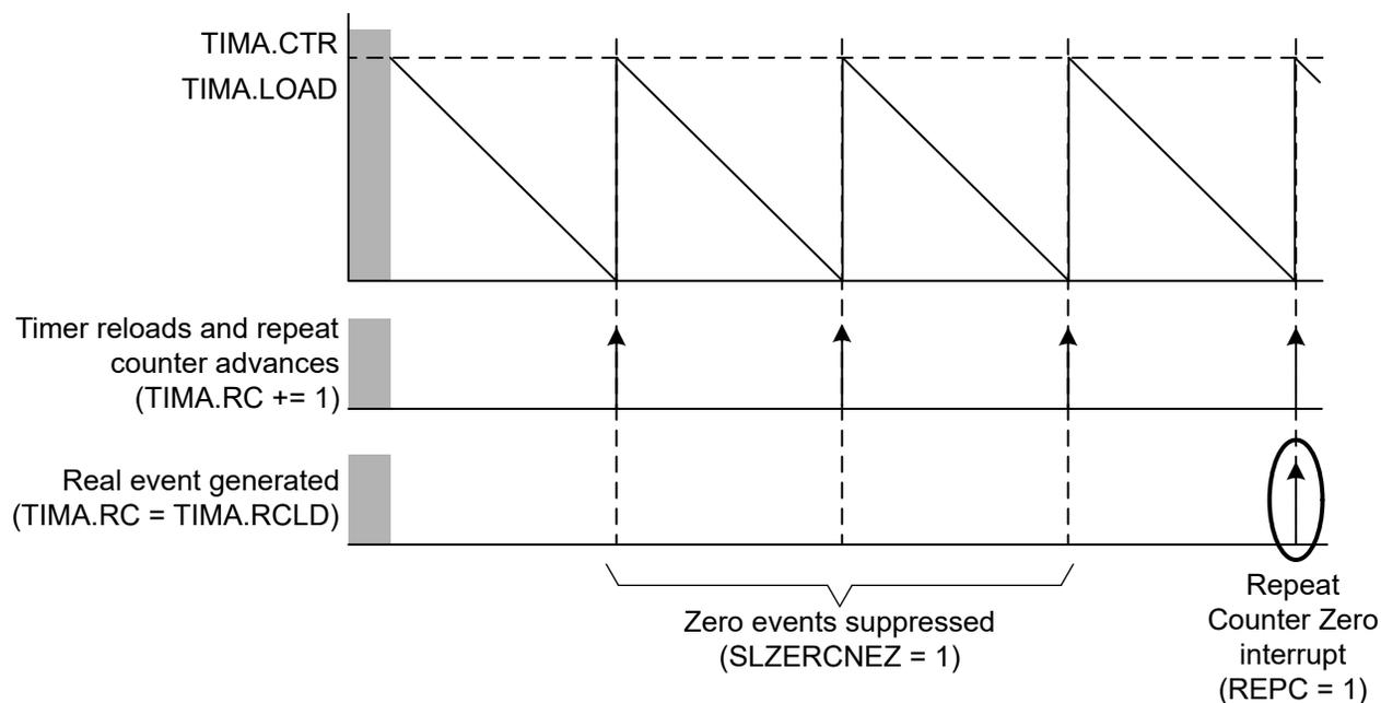
**Figure 23-3. Event Suppressed by Repeat Counter with TIMx.RCLD = 4 in Down Counting Mode**
