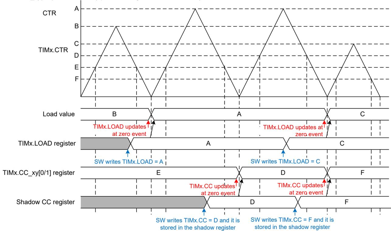
Figure 23-25. Shadow Load and Shadow Compare Taking Effect at Zero Event in Up/Down Mode
