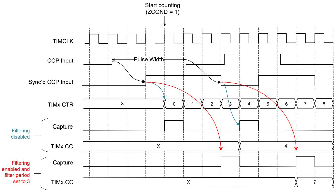
**Figure 23-16. Pulse-Width Capture Mode**
