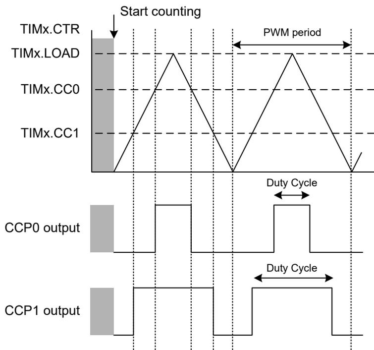
**Figure 23-30. Center-Aligned PWM**
