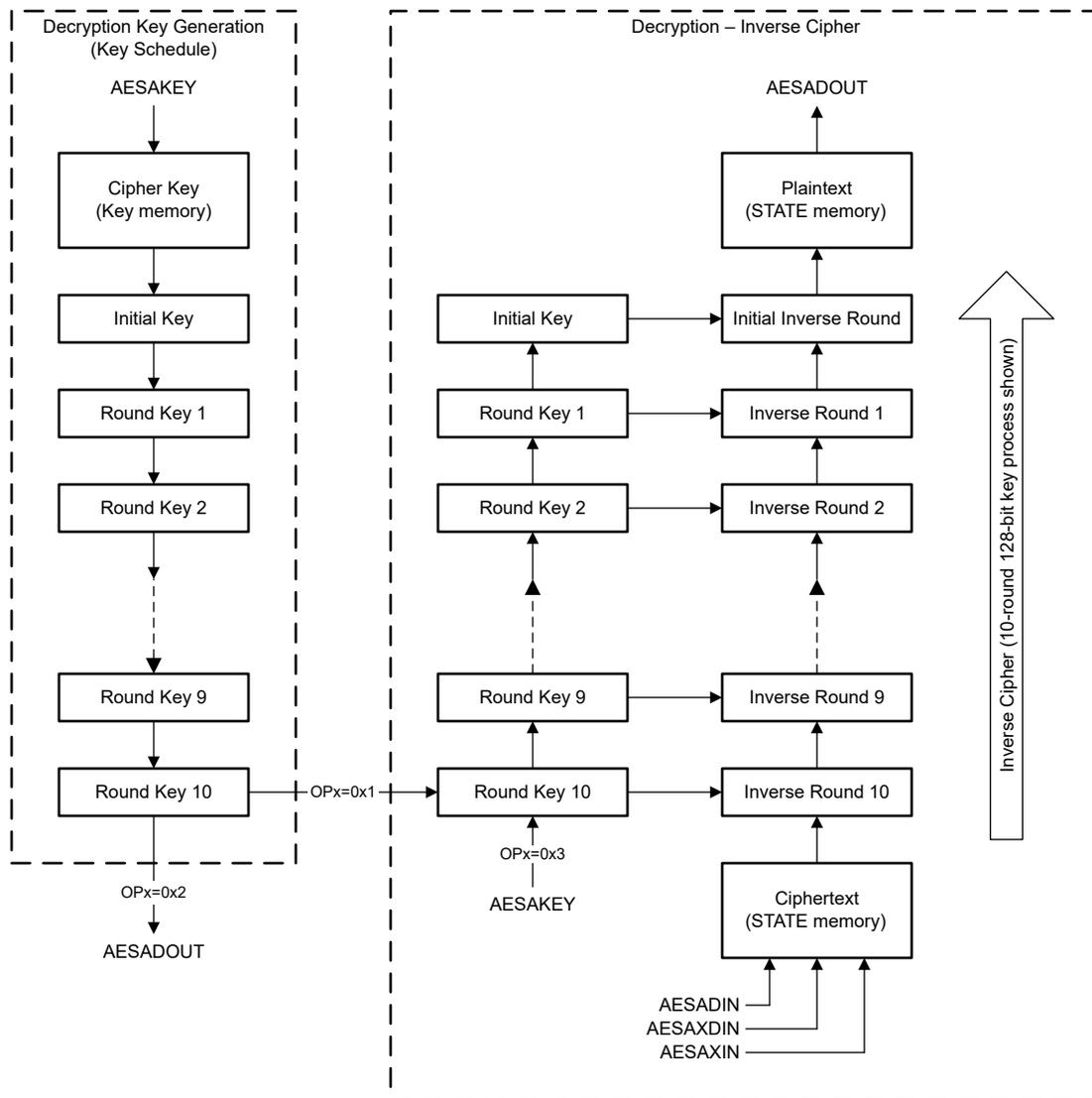
**Figure 21-4. AES Decryption (OPx = 0x1, 128-bit Key)**
