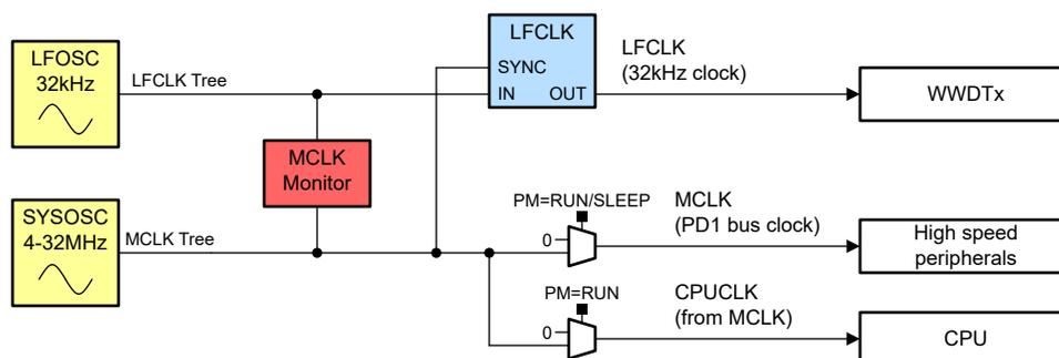
Figure 25-3. WWDT Simplified Clock Source Tree
