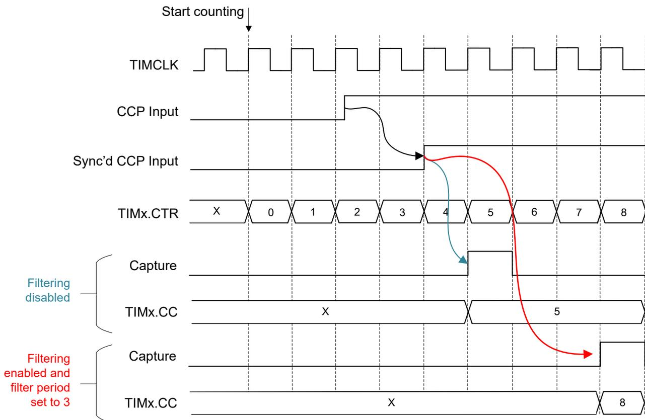
Figure 23-14. Edge Time Capture Mode in Up-Counting Mode,  $CVAE = 2$
