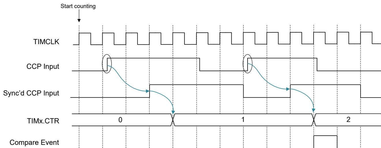
**Figure 23-23. Edge Count Operation to Generate Compare Event (TIMx.CC = 2)**
