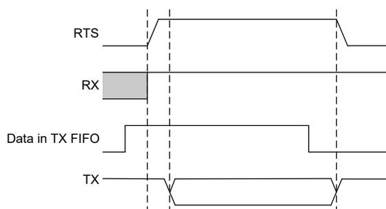
**Figure 16-10. RS485 Data Exchange**
