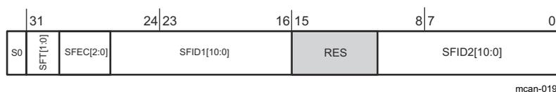
**Figure 19-24. Standard Message ID Filter Element Structure**
