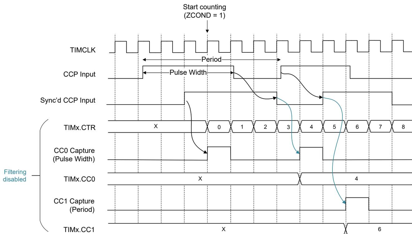
**Figure 23-17. Combined Pulse-Width and Period Capture**
