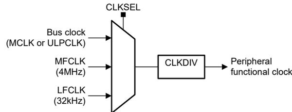
**Figure 2-9. Peripheral Clock Selection Mux and Divider**
