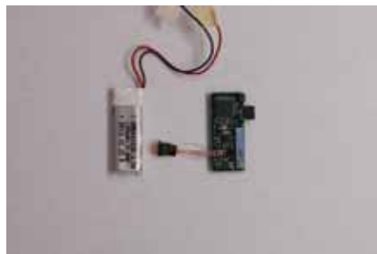
Fig. 4 The embedded device contains a microcontroller, wireless transmitter/receiver, antenna, analog circuits, and a battery.
